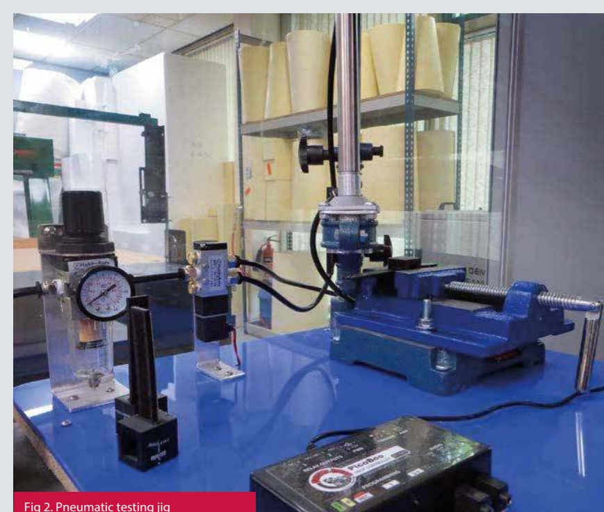
Fig 2. Pneumatic testing jig
